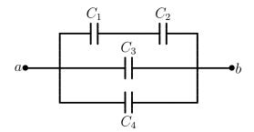
Four capacitors are connected as shown above. Each capacitor has a capacitance of  $4.0\mu F$ . A voltage of 10V is applied between the points a and b.
