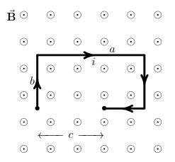
The figure above shows a magnetic field  $\vec{\bf B}$  directed out of the page. Its magnitude is 3.0T. A piece of wire is placed in this magnetic field in the plane of the page as shown. The top segment has a length  $a=4.0{\rm m}$  and the left segment has a length  $b=2.0{\rm m}$ . The distance between the ends of the wire is  $c=2.5{\rm m}$  A current of  $i=5.0{\rm A}$  is flowing in the wire in the direction shown.
