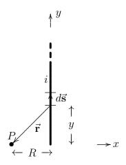
A long thin wire is bent in the shape shown above. Assume it extends to infinity in the positive y and positive x directions as shown. A current i flows in the wire as shown. The point marked P is at a distance R along the negative x axis as shown.
