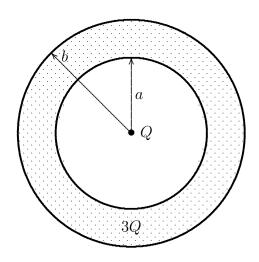
The figure above shows a conducting spherical shell (inner radius a and outer radius b). It has a charge of 3Q placed on it. A point charge of Q is placed at the center of the sphere. Q is positive. The system is under static conditions.
