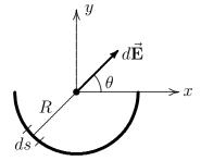
The figure above shows a thin wire bent in the shape of a half circle of radius R with center at the origin of the coordinate system shown. It has a uniform charge density of  $\lambda$  C/m. Other symbols to be used are shown in the figure.
