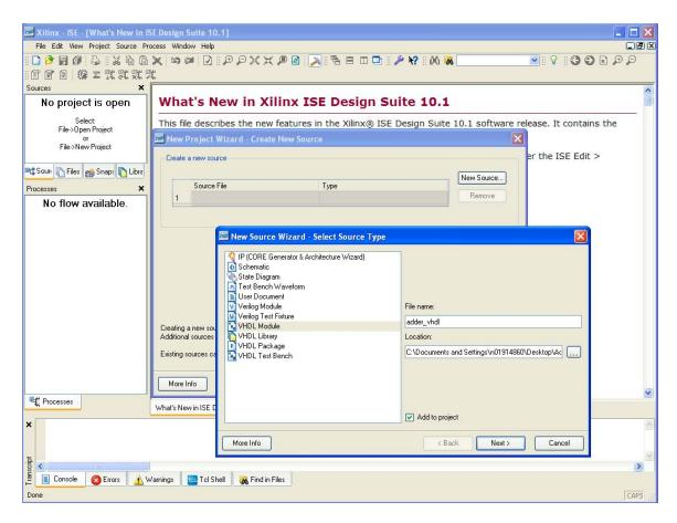
Click "Next". In this exercise, you are designing a full adder with x, y, and z as inputs and s and c as outputs. Hence, set the ports accordingly and click Next.
