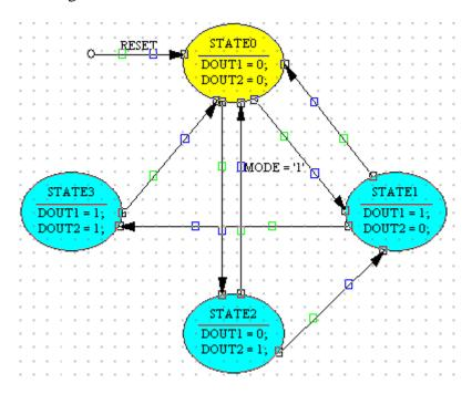
Finish the diagram by applying the following conditions and outputs for each transition:
