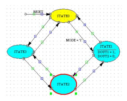
Alternatively, you may type the value of the output for a given state; no need to run the "Output Wizard". Double click State2. Edit the outputs as seen below. Click "OK" when done.
