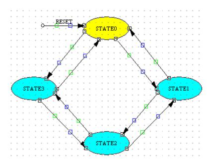
Now that the basic diagram is in place, we need to add/remove/modify the current transitions to obtain the correct state diagram for the sequence generator. Left-click on one of the two boxes of the transition arrow **State0-->State1**. This will bring up the "Edit Conditions" dialog box. Add the condition **MODE** = '1' in the "Conditions" box.
