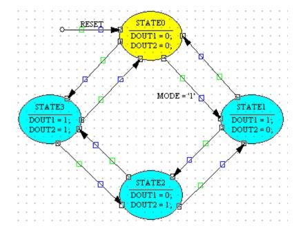
If a state transition is not needed, it can be deleted by left clicking on the transition line and pressing the delete key. Let's delete the following state transitions.
