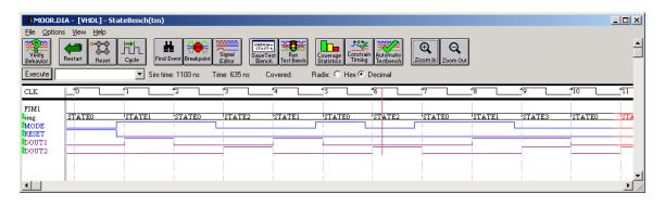
Verify that your design is correct by viewing the generated waveform.
