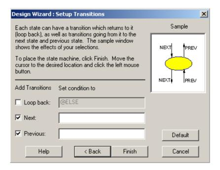
The template state diagram has been created but it still needs to be placed onto the blank diagram window. To place the diagram created from the wizard, left-click anywhere on the blank diagram; an inch from the top-left corner is a good place.
