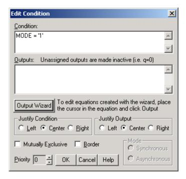
This condition will make the transition **State0-->State1** occurs when **MODE** is true or '1'. Click "OK". Your diagram will now have the condition on the transition line.
