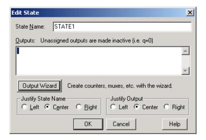
To assign the correct output for that state, click on the "Output Wizard" button. Select "Constant" from the upper left box, type 1 in the "CONSTANT" box, type DOUT in the "DOUT1" box, and set the "Data path width" to 1. Click on "OK".
