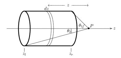
Consider the axis of the solenoid to be the z axis with its origin at the target point P. Approximating the packing of the wires to be continuous, the current in a thin ring of thickness dz is In dz. So the magnetic field due to it is given by equation 5.41 (example 5.6) to be
